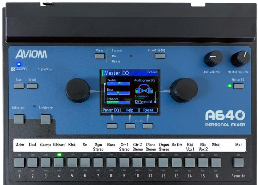
*The Audiogram EQ user interface uses two simple, intuitive controls to adjust the amount of correction applied.*
